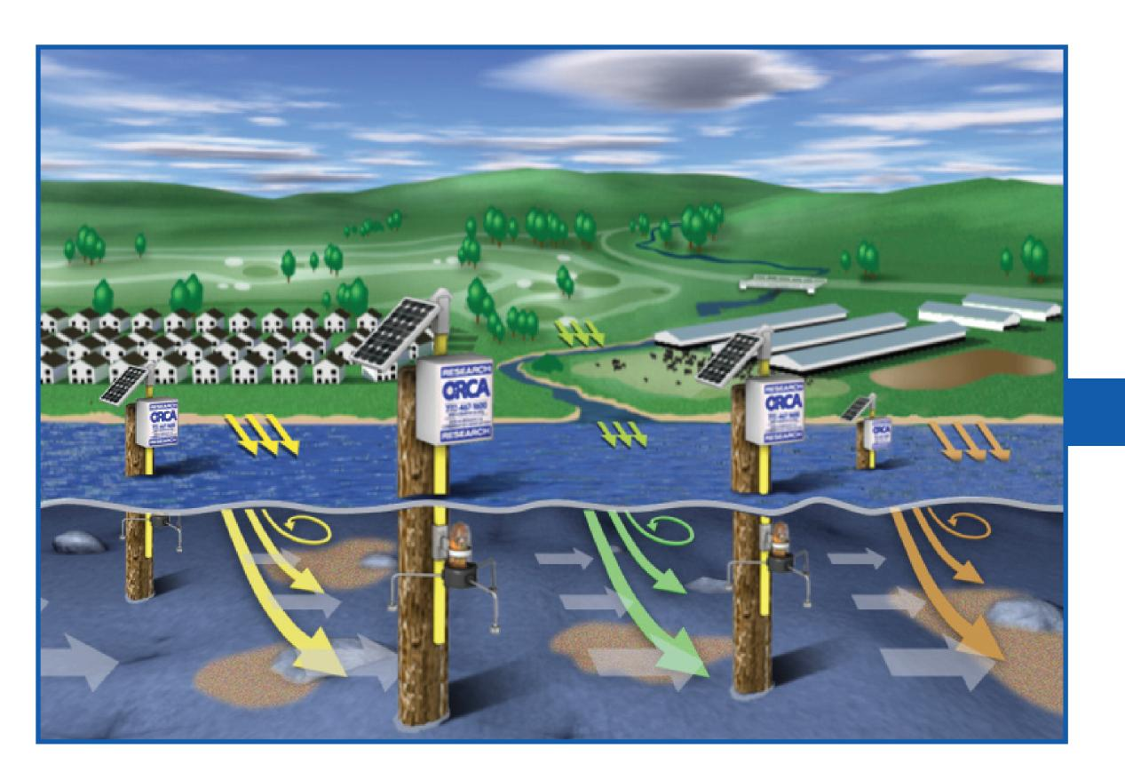
The ORCA Kilroy Network consists of a wireless network of remote semiautonomous sensor systems. This is coordinated by a central supervisory system that directs operations of the remote systems, collects data, and relays them via the Internet through a standard web service interface to a geospatial database in near real time. The coordination and data transfer are presently over cellular Internet connections on a wide scale and cabled connections at the station scale.
